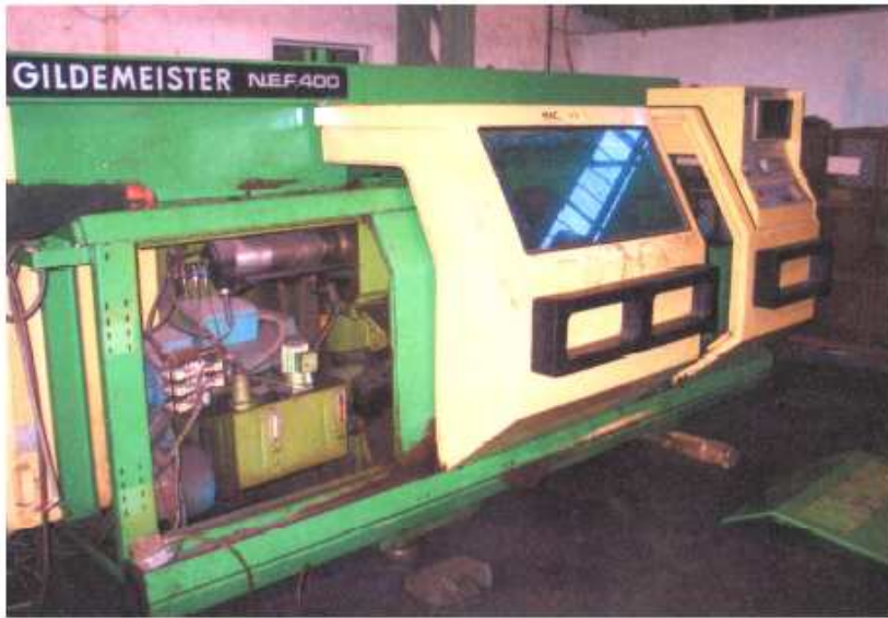
Manual Tailstock Converted to Hydraulic
