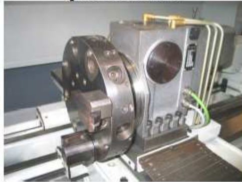
The original Turret disk fitted to High speed Servo Turret
