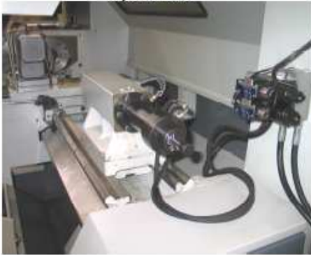
Manual Tailstock Converted to Hydraulic
